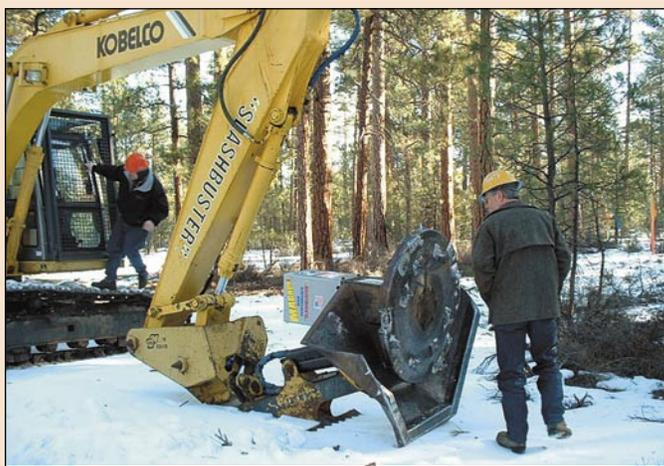
Figure 1. Slashbuster equipped with rotating head.
